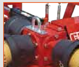
Heavy duty center-splitter gearbox
