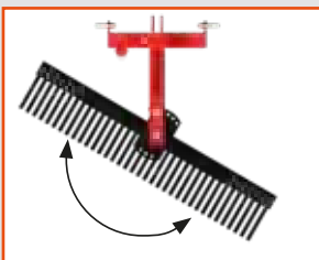
Up to 32° angling on standard duty rakes
