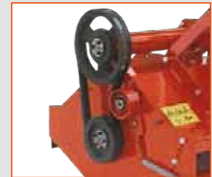
Double belt transmission with automatic belt tensioner
