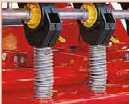
Precise seed metering cups
