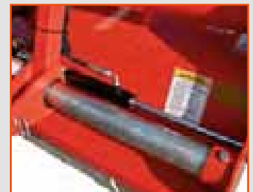
Hydraulic cylinder for side shift
