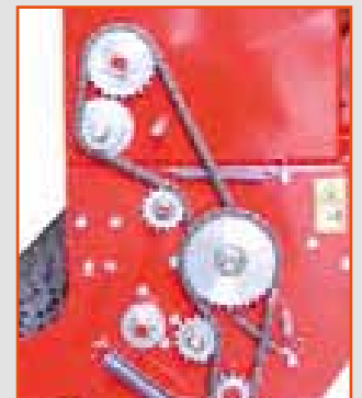
Seed distribution engaged by ASA 50 chain transmission
