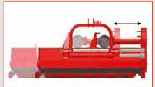
Manual or hydraulic side-shift up to 16"
