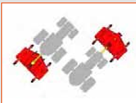
Reversible hitch for front or rear mounting
