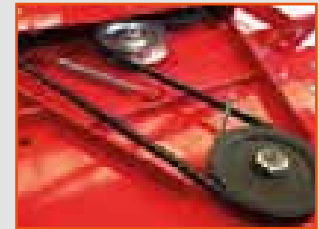
Heavy duty reinforced belt (BX) with automatic belt tensioner
